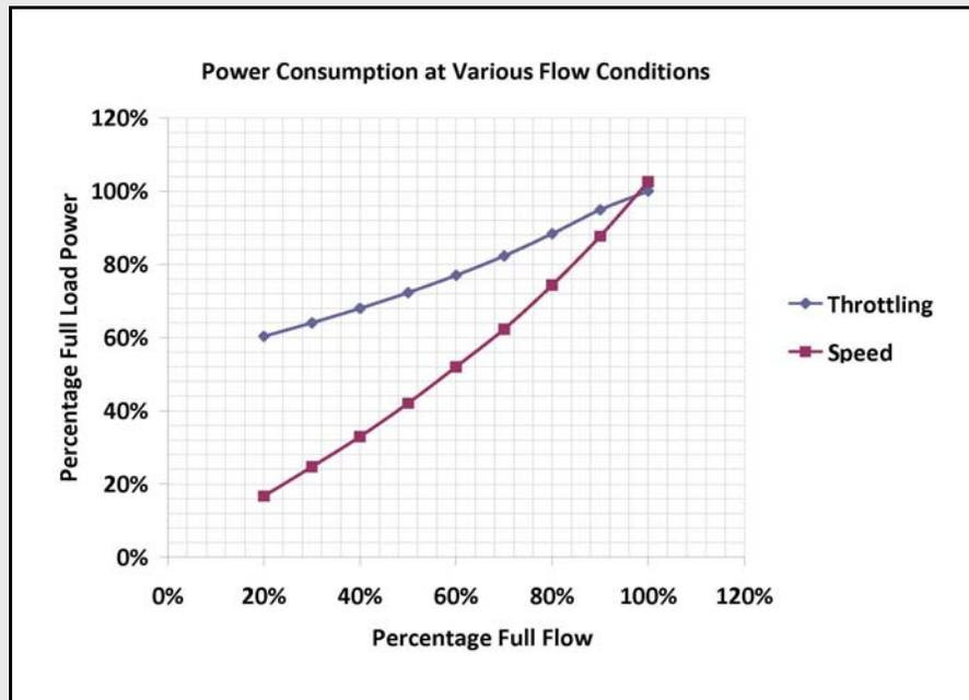
During events of low demand, VFD control will not be as effective. A fundamental limitation of VFD is the minimum speed at which it can operate. If the system demand falls below this minimum speed requirement, the pumps must operate as if there were no VFD control in place (although this situation may happen less than 20% of the time the pump is operational.) Typical savings achieved are upwards of 10% of pumping energy.
