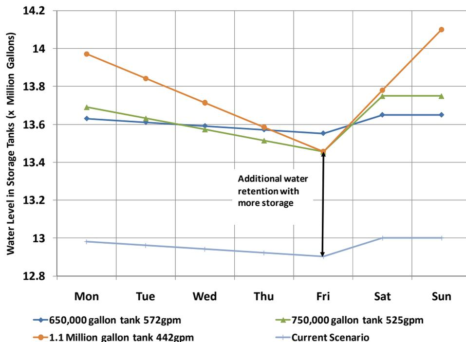
If the water utility's minimum acceptable storage capacity is 13.5 million gallons, the energy audit of this system may recommend capacity upgrades as well as optimized use of existing pumping and control systems to achieve a savings of as much as 20% of the total energy consumption.
